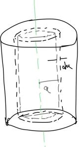
Many of the hollow against - $\frac{M}{HR^2L} \left(2\pi n\right) dn. L = \frac{2M}{R^2} l. dn$  $dT = \int \frac{2M}{R^2} \cdot n \cdot dn \int \cdot n^{-1}$ Theer, the moment of Treating of the Solid against is,  $J = \int \frac{2M}{R^2} n^3 M = \frac{MR^2}{2}.$ I The farmular down not defeat our the beight of they afterder. Moment of Insertion of an uniform below below about a liameter - May M, Rodina R. PAD DAR O May per unit area of the Sphere = M 4TTR2
